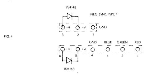
CURE 3: Join negative sync inputs J2 and J3 together with a jumper. Locate W102 and install a jumper from W102 to either J2 or J3.
