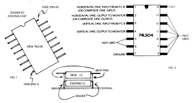
CURE 2: Used for Wells-Gardner Video-Sync boards with positive sync connections only. (Vertical mount board 85×140B.
