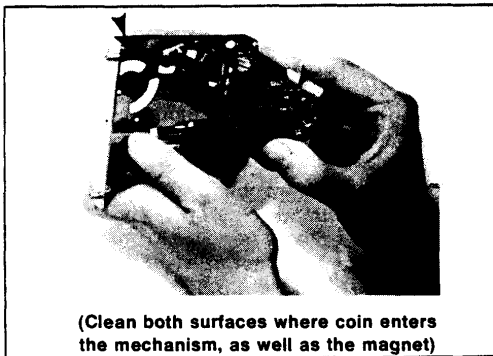
Figure 3-4 Surfaces to Clean Inside the Coin Mechanism
