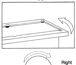
When the trackball is rolled to the right the table should spin counter clockwise.
