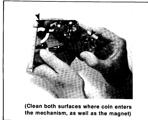
Figure 9 Surfaces to Clean Inside the Coin Mechanism
